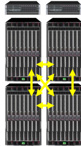
64S Cabled (4xB16) 32 Blades (36U, dual 19" racks)
