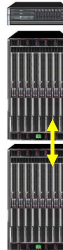
32S Cabled (2xB16) 16 Blades (36U, 19" racks)
